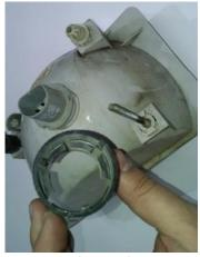
Make note of the orientation of the collar and its fingers for reinstallation.
