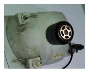
7. Check emitters are facing left and right once inserted into light housing.
